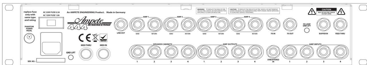
10. **FX IN:** Connect the FX IN jack of the 444 to the input of your effect, whether it is a single unit like a delay pedal, a chain of pedals or rack units or another audio looper. This is exactly like you would connect it to your amp's FX Loop Send. When switching between amps on the 444, it automatically switches your effects to the currently selected amp.
